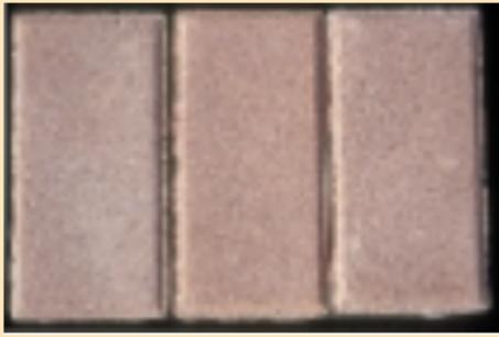
Completely eliminating the chance of efflorescence, however, isn't possible because it's a natural byproduct of hardened concrete. It will stop when no more calcium hydroxide is available to move to the surface.
